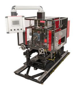
Our Lancer is a mechanical device that works inline with pour and debridge processing machinery to prepare and condition the thermal barrier pocket in our aluminum extrusions prior to the polyurethane polymer filling step.
